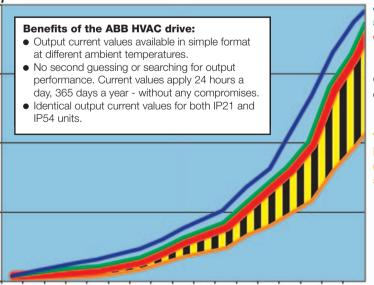
4 5.5 7.5 11 15 18.5 22 30 37 45 55 75 90 kW The figure shows output currents of the ABB HVAC drive at ambient temperatures of 40 °C and 50 °C. The thick red curve illustrates the required nominal motor current of ABB M2000 range eff2 motors, while the orange curve shows the output current of a typical drive (other than ABB) in the market.
